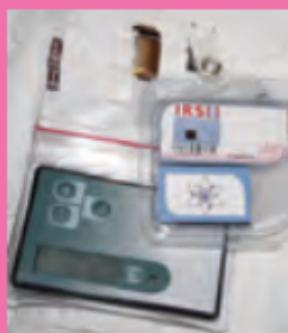
Radioactivity can't be felt. Special measurement devices are needed to quantify radioactivity. A dosimeter measures a worker's exposure to the radiation.
